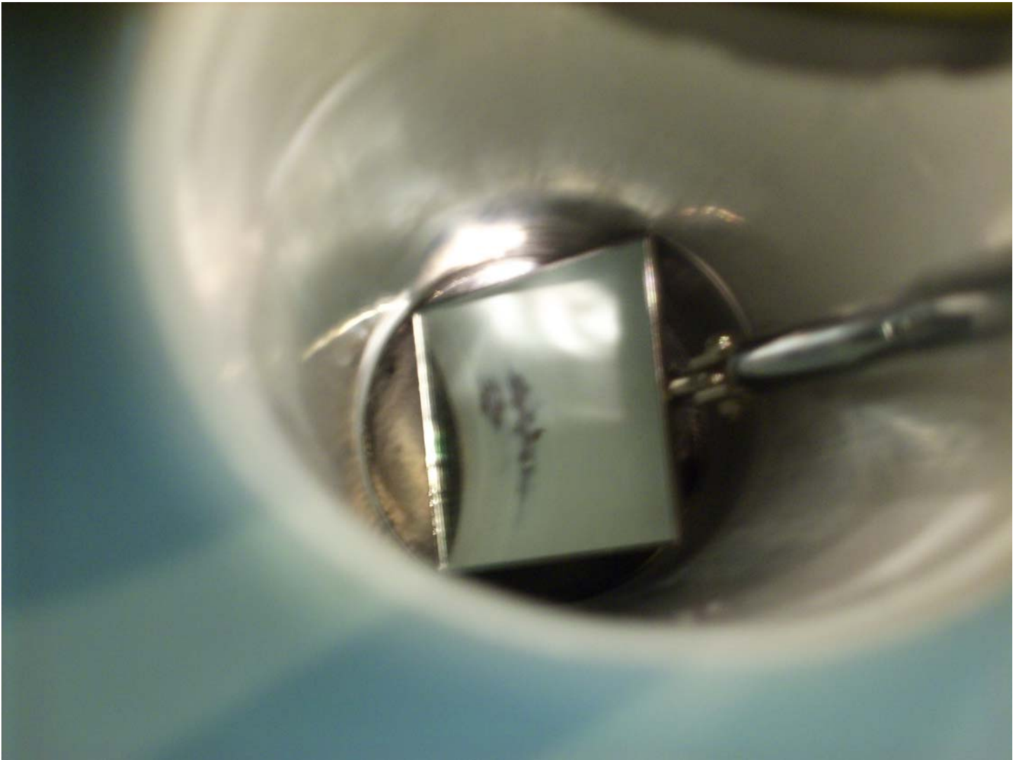
Figure 2: Mirror shows (somewhat) the rubbed off gelcoat on the front,bottom wall of the mast well. For now, just the gellcoat has been work off in this area. I am looking for a way to reseal, recover this worn area to prevent water from seeping/leaking into the now exposed fiberglass.
