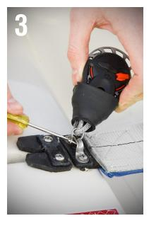
Tighten the shackle with a screwdriver making sure that the shackle is positioned with the pin at the bottom against the saddle.
