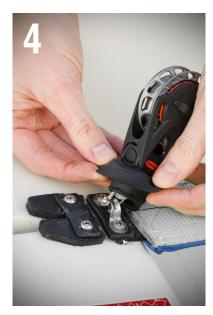
Roll down the boot and align it over the saddle.
