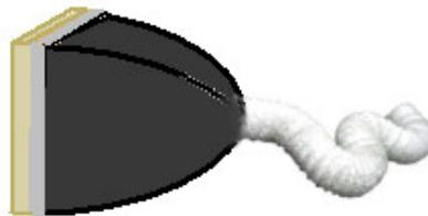
With a single port, fan-forced air can be piped in using a shop-vac hose or a small dryer vent hose so long as the hose size leaves enough room through the inspection port for exhaust air to exit around it. A dual port, fan forced system gives the best outside air exchange.
