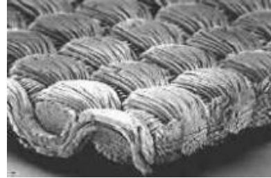
Magnified view of tightly woven Dacron® Polyester.
