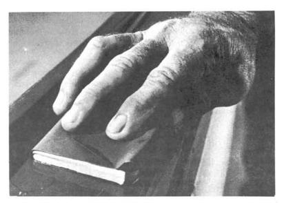
USING A SANDING BLOCK, sand the patched area with 600 grit WET sandpaper. Finish by rubbing or buffing with a fine rubbing compound. Some slight color difference may be observed. Weathering will blend touch-up, if properly applied.
