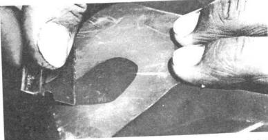
11. Immediately after trimming, place another small amount of gel coat on one edge of the patch and cover with cellophane. Then, using a rubber squeegee or back of the razor blade, squeegee level with area surrounding the patch. Leave cellophane on patch for 1 to 2 hours, or overnight, for a complete cure.
