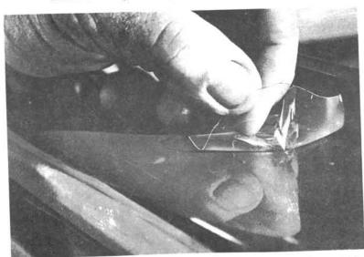
(5) Lay a piece of cellophane or waxed paper over the repair to cut off the air and start the "cure."
