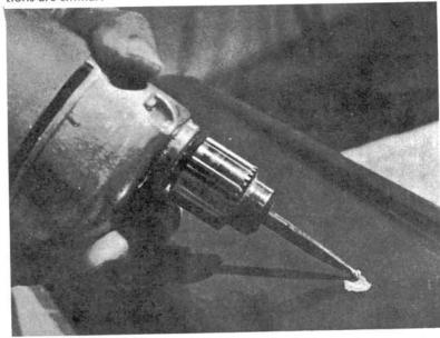
For damage to the gel coat surface, you will need a small can of gel coat, of the same color as your boat, and a small amount of catalyst. For deeper holes or gouges (1/8" or more) you will also need some short strands of fiber glass which can be trimmed from fiber glass mat or purchased in the form of "milled fibers." These materials can be purchased from your dealer.
